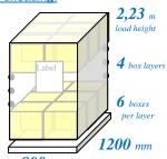
800 mm Articles in a pile: 50 Piles in a box: 16 Articles in a box: 800 Box inner size: 392x392x510 Box load gross: 5,23 kg Boxes per pallet: 24 Articles per pallet: 19200 Pallet height: 2,23 m
